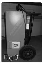
The operating position requires the folding support leg to be folded down and secured into position by the locking rings.
