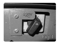
Fit correct plug top to power input lead to suit operating voltage selected.
