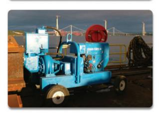
Performance Max head: 38m, Max flow: 90 l/s, Max solid: 52mm
