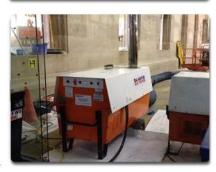
Power supply 230/110 V 1 ph 50 Hz Run 6.2/15.1 A
