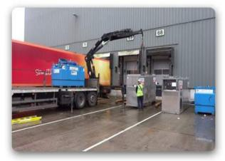
Power supply 415 V 3 ph +E 50 Hz Run 20 A Nominal Heating 383 kW 1,306,796 btu Generator size 20 kVA Noise level (max) 76.5 dBA @ 1 metre Duct size 600 mm x 2 Weight 1300 kg Fuel Consumption 38 ltrs/hr Dimension 3,850 x 1,200 x 2,015 mm Typical heated area 8,457 m Control Manual, External controls available (24 V external control circuit) Fuel type Gas Oil Plug type BS4343 4 pin 3 ph 32 A Flue 1 mtr x 250 mm
